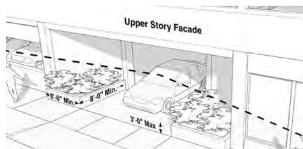
2. In the sight triangle, defined as the area bound by the parking structure wall, sidewalk, and driveway; landscape or a solid masonry wall, a maximum of three feet in height, must be included to act as a buffer between the driveway and sidewalk.
