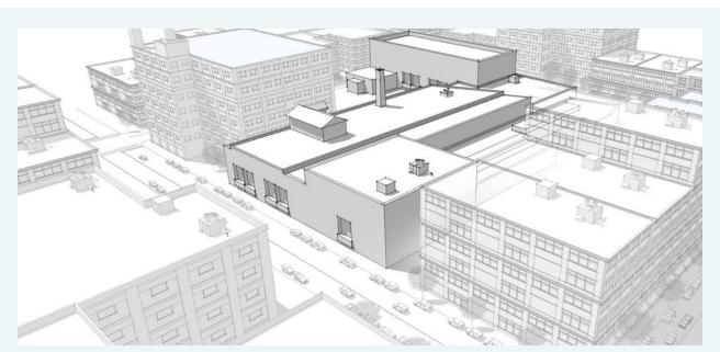
An industrial shed is a single-story structure with a large footprint, often naturally lit with monitor or sawtooth roofs. Such structures are typically designed for industrial, office, or "big box" retail uses.
